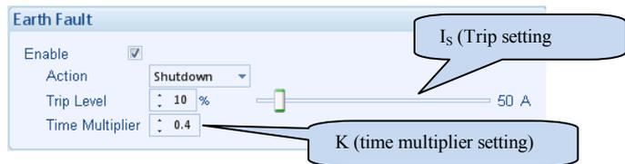
The settings shown in the example above are a screen capture of the DSE factory settings, taken from the DSE Configuration Suite software.
