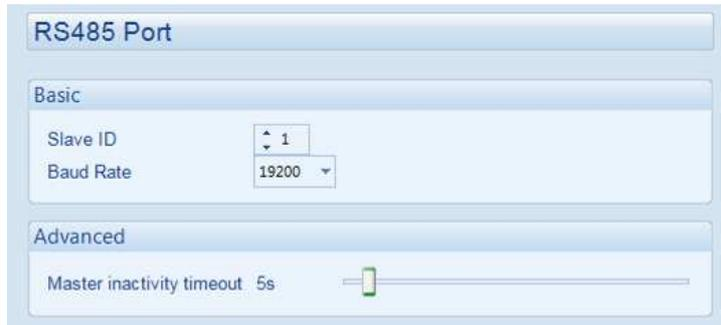
'Master inactivity timeout' should be set to at least twice the value of the system scan time. For example if a modbus master PLC requests data from the module once per second, the timeout should be set to at least 2 seconds.
