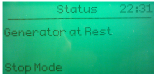
Factory setting of Status screen showing engine stopped...
